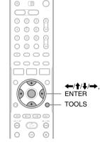
1 Before recording starts, press TOOLS to select "Rec Settings," and press ENTER.
